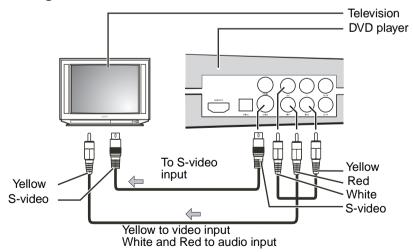
If the TV has an S-video input, connect the player with an S-video cable. When using an S-video cable, do not connect the yellow video cable.
